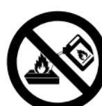
Never fill liquid fuel into the Bio-Burner while it is burning!
