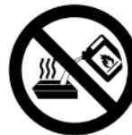
Never fill liquid fuel into the Bio-Burner while it is hot!
